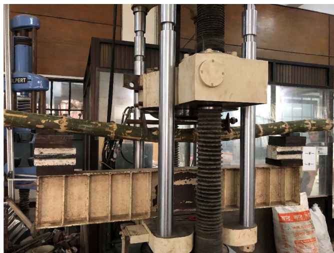
Fig. 12. Bambusa tulda sample being tested for bending strength.
