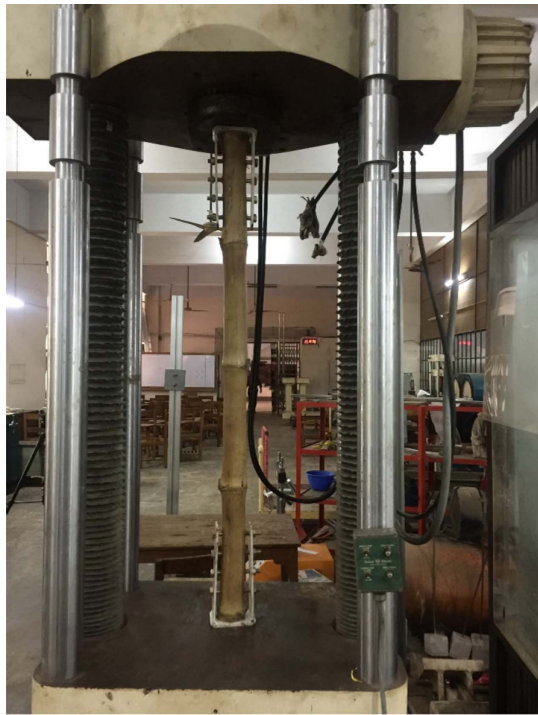
Fig. 7. Bamboo sample in universal testing machine.
