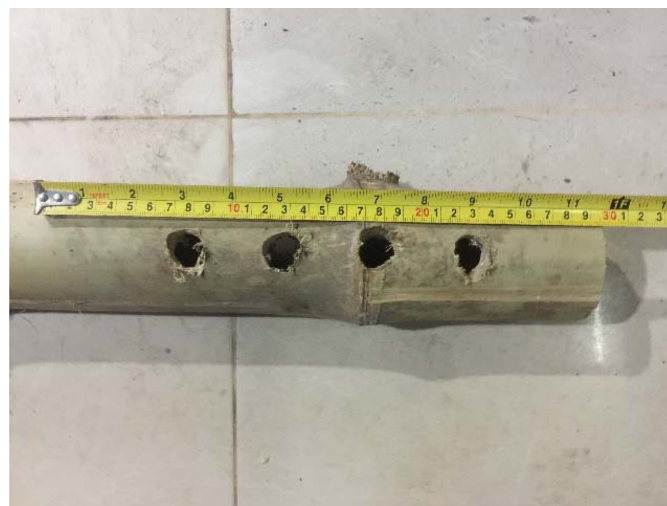
Fig. 3. Drilling holes at bamboo end for inserting 12-mm bolts.
