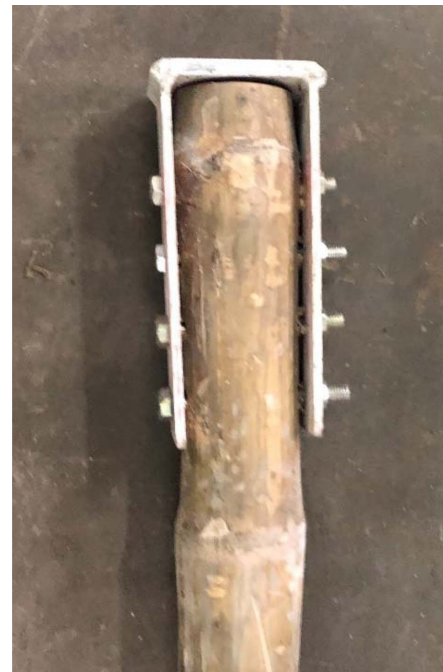
Fig. 6. Mild steel joint system attached to bamboo ends.
